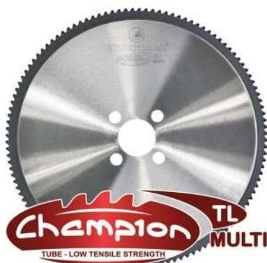
A dedicated Champion TL Multi saw blade has been developed for multiple tube cutting with a tensile strength of 400 – 800 N/mm<sup>2</sup>. This blade type is specifically suited for Rattunde Twin machines but also for other applications where multiple tubes are being cut, such as the BEWO, RSA and Sinico machines.
